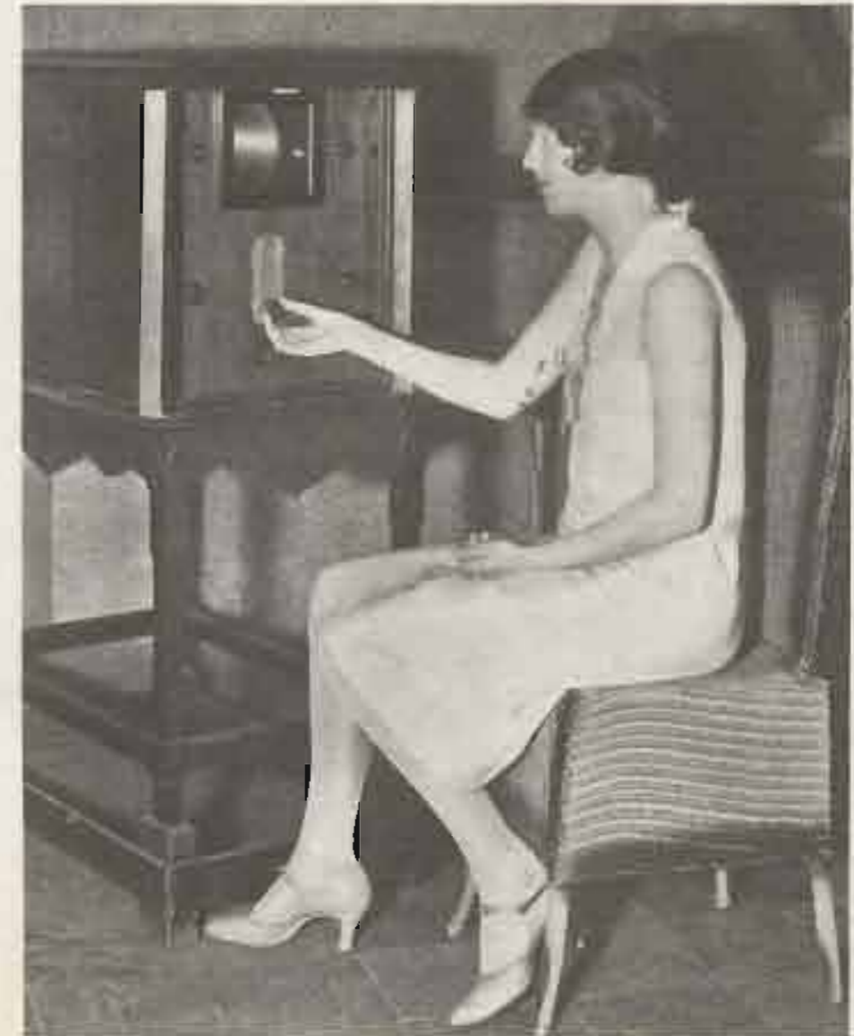
Television receiver. Picture is three inches square and has a pale, pinkish glow.
